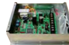
Relay Interface BMS-IFLSV4E For TCS-NET
